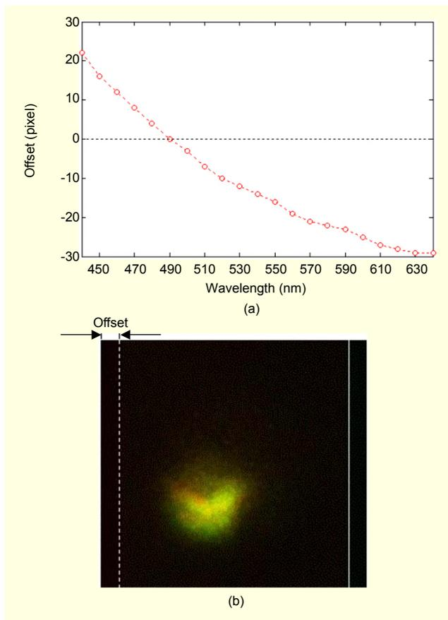
Fig. 3. (a) The amount of spatial offsets of spectral band images caused by the AOTF with respect to the reference band at 490 nm and (b) registered band images of 490 nm and 540 nm.
