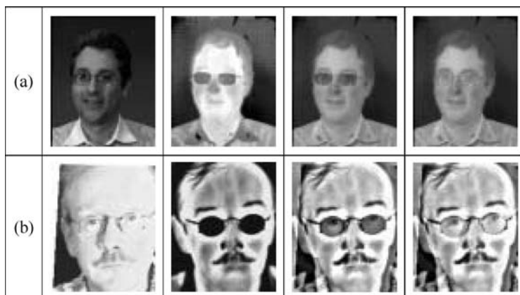
Figure 13. DWT-based image fusion with eyeglass replacement for image samples from (a) NIST/Equinox database and (b) UTK-IRIS database. From left to right are: Visible image, Thermal image, Fused image without eyeglass replacement, and Fused image after eyeglass replacement.
