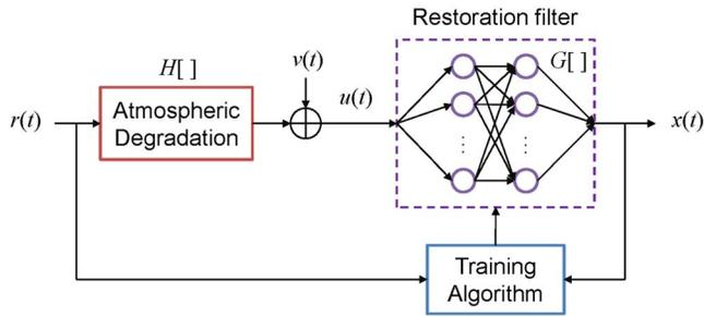
FIG. 4. (Color online) Training of the terahertz restoration filter based on artificial neural networks.
