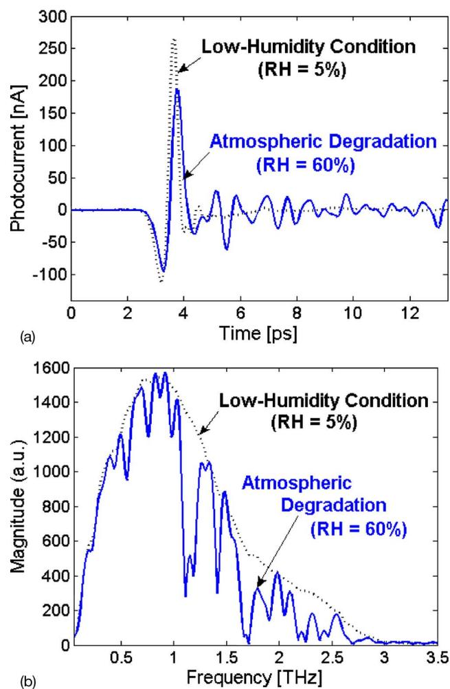
FIG. 2. (Color online) The effects of atmospheric degradation in terahertz spectroscopy signals: (a) time waveforms and (b) Fourier spectra.
