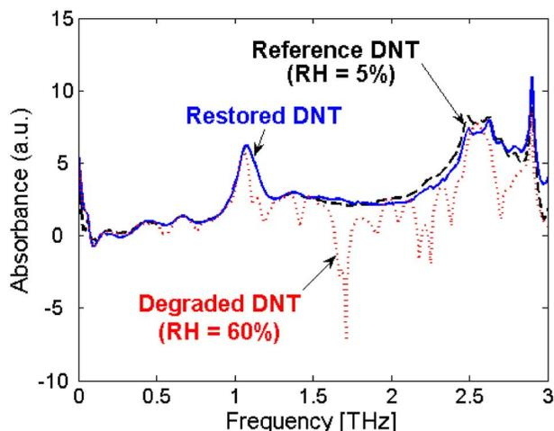
FIG. 9. (Color online) Restoration of terahertz signals from atmospheric degradation.
