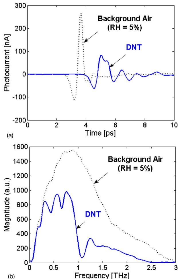
FIG. 6. (Color online) Terahertz signals of background air and a DNT sample measured in low-humidity conditions: (a) time waveforms and (b) Fourier spectra.
