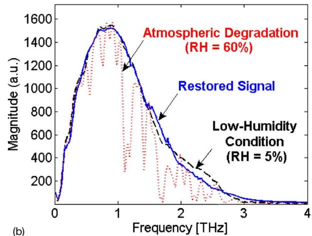
FIG. 5. (Color online) Restoration of terahertz signals degraded by atmospheric propagation: (a) time waveforms and (b) Fourier spectra magnitudes.
