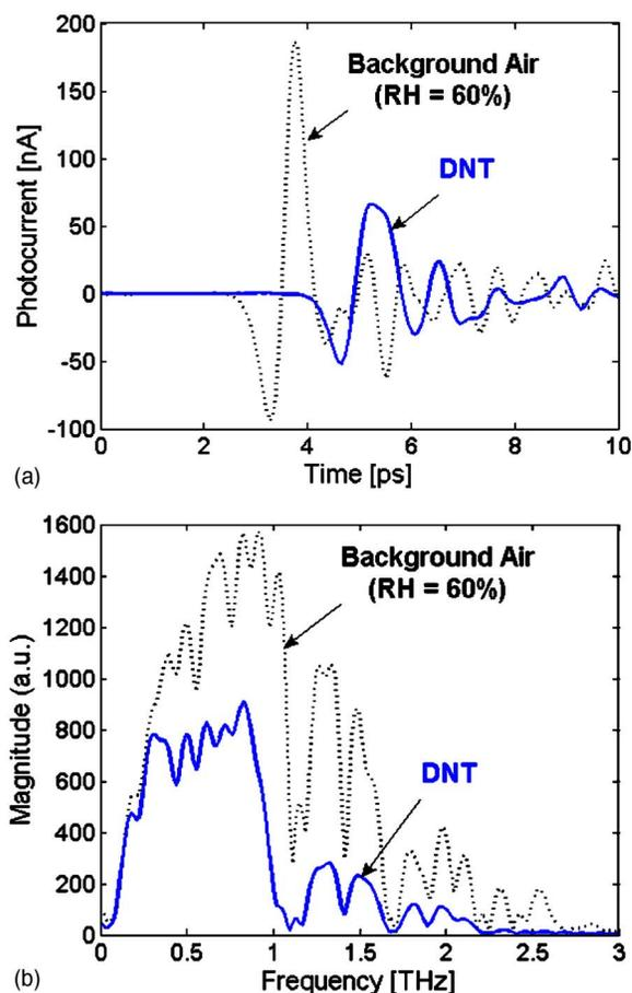
FIG. 7. (Color online) Terahertz signals of the background air and a DNT pellet, measured in an open-air environment at 60% humidity: (a) time waveforms and (b) Fourier spectra.
