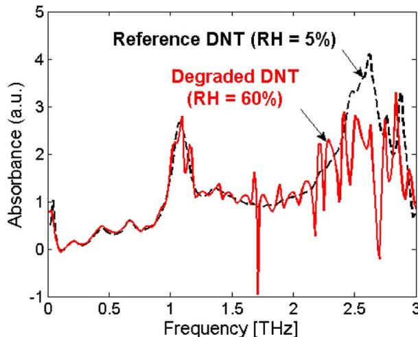
FIG. 8. (Color online) Absorption spectra of DNT measured at low-humidity and humid open-air conditions.
