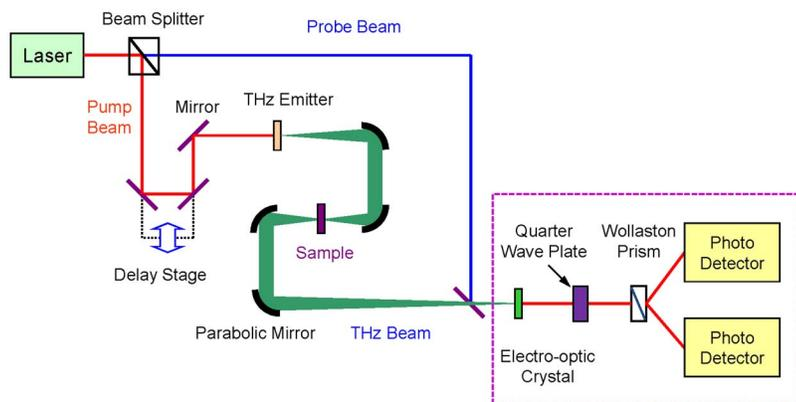
FIG. 1. (Color online) A schematic diagram of the time-domain terahertz spectrometer.
