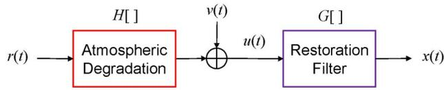
FIG. 3. (Color online) Restoration process for degraded terahertz signals.
