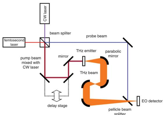
Fig. 1 THz-TDS with CW laser mixed with femtosecond pump laser beam
