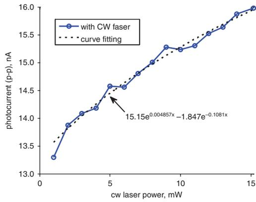
**Fig. 5** THz radiation power improvement against CW laser power
