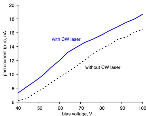
Fig. 3 Increase in THz radiation as bias voltage changes
